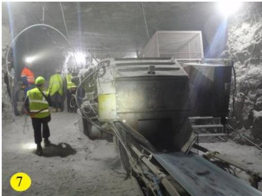
Turning another corner the conveyor end is found where loose material is pushed onto a short belt which feeds lumps of rock into a crusher (**Pic 7**) where they are broken down to more manageable size for the conveying system. The crusher comprises two revolving steel drums with hardened teeth that do the breaking up as the rock meets them and is pushed in.
